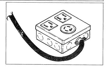
A 240 volt, 4-prong, 20 amp connector plug is included with the alternator. If additional plugs are required, refer to REPAIR PARTS section of Owner's Manual. The 240 volt outlet will supply both 120 volts a-c and 240 volts a-c, as shown above, when a 4-wire cable is connected to the connector plug.
